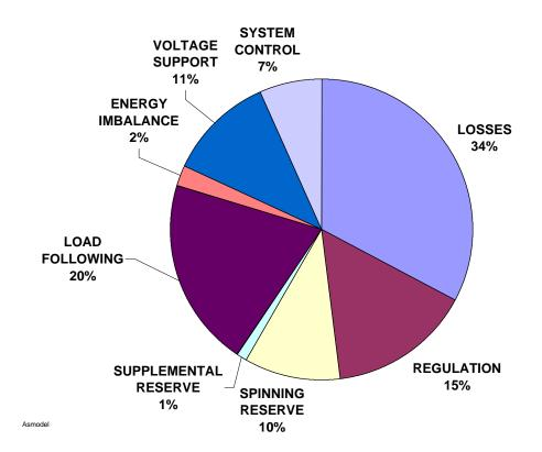
Figure 4-1. The allocation of ancillary-service costs for a hypothetical system. (In total, these services cost the equivalent of \$2.3/MWh during the course of a year.)
