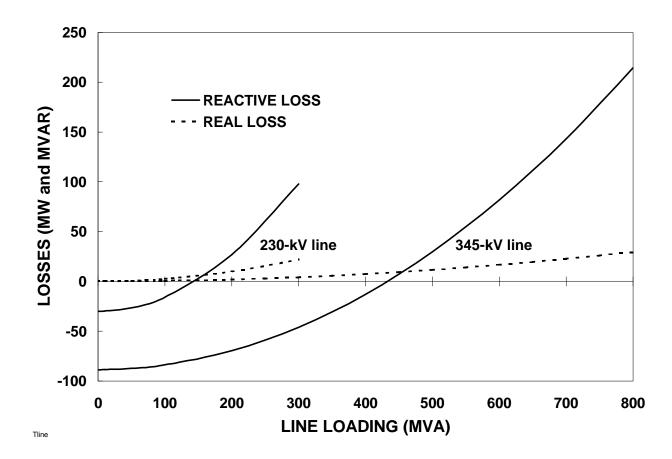
Figure 7-1. Transmission lines supply reactive power to the system when lightly loaded but absorb reactive power when heavily loaded. (These results are for a 100-mile line with voltages supported at both ends.)
