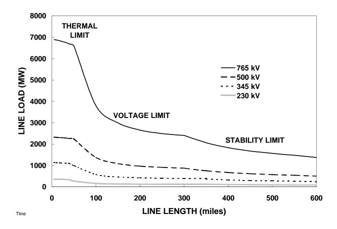
Figure 7-2. Absent reactive compensation to maintain voltages, transmissionline capacity is limited to shorter lengths.
