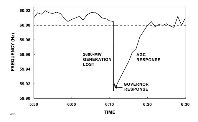
Figure 5-1. Interconnection frequency before and after the loss of a 2600-MW generating unit.
