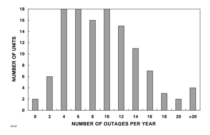
Figure 5-2. Number of forced outages in 1996 for 120 coal-fired generating units between 600 and 800 MW in size.
