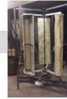
VAWT Generator 1-50 kW
