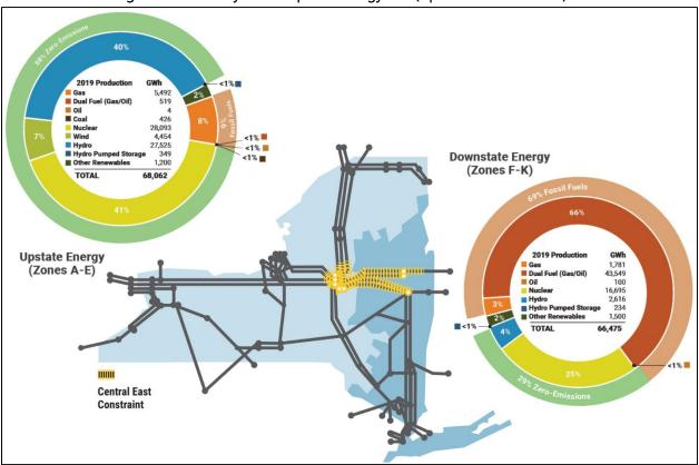
Figure 11: NYISO System Map and Energy Mix (Upstate vs. Downstate)<sup>46</sup>
