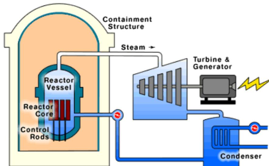
The boiling water reactor (BWR) was designed by General Electric (GE-Hitachi) to compete with Westinghouse’s PWR design. Advantages to the BWR include operating at a lower pressure removes the need for a high pressure reactor vessel and direct transfer of reactor steam to the steam turbine eliminates the need for the steam generator found on PWRs. One drawback is that BWR operators are exposed to higher radiation levels.
