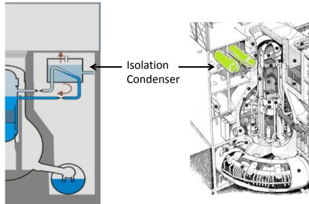
It is possible that the Unit 1 ICs were damaged during the earthquake; however, 11 minutes after Unit 1 shut down due to the earthquake and prior to the tsunami, the reactor operator manually stopped both trains of the IC cooling.<sup>171</sup> TEPCO officials told the Independent Commission that this was the first time the IC system had automatically started and ever been used since the plant started operation in 1971.<sup>172</sup>
