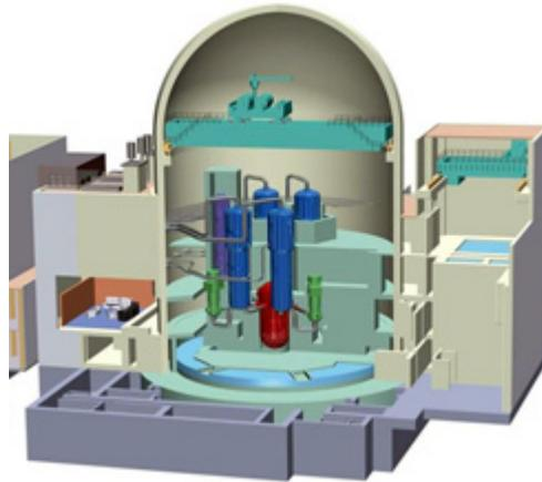
A four-train redundant safety system provided to enhance safety and improve reliability. NRC design certification for the U.S. APWR is underway and currently projected for completion in 2015. In the meantime, both Dominion Energy (North Anna) and Luminant (Comanche Peak) have COL applications before the Nuclear Regulatory Commission.<sup>228</sup>
