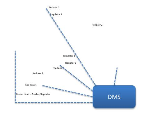
**Conservation of Voltage Reduction (CVR):** A voltage reduction scheme that flattens and lowers the distribution system voltage profile to reduce overall energy consumption.
