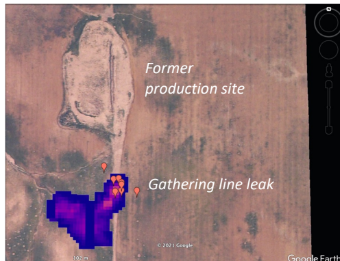
Methane plume images fused with high resolution context camera image
