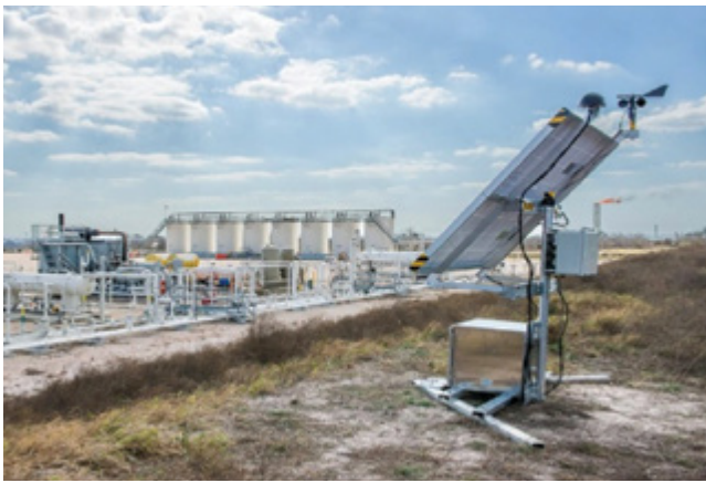
Quanta3 Continuous Methane Detection System being field tested at Statoil
