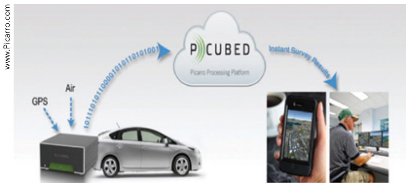
A working diagram of the Picarro Surveyor
