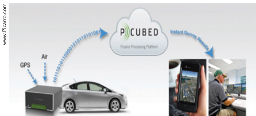
A working diagram of the Picarro Surveyor
