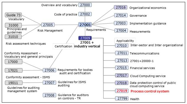
Figure 7: ISO/IEC 27000 Series, Identifying 27019 Specifically for Process Control Systems Source: ISO/IEC 27000 series, [8]
