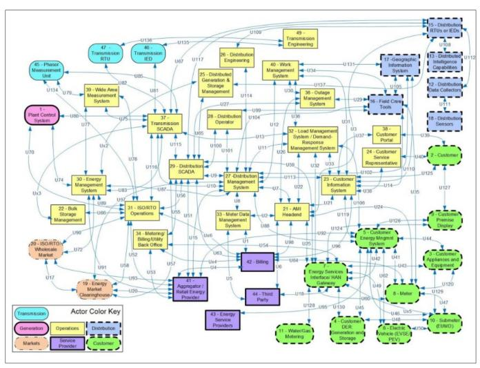
Figure 11: NISTIR 7628 Spaghetti Diagram High-Level Logical Reference Model Source: NISTIR 7628, [17]
