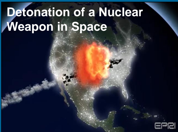
E1 – Fast Pulse (50 kV/m - 2.5 nsec rise time)
