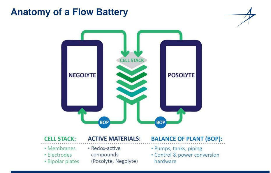
Flow batteries decouple power and energy, lowering marginal cost of multi-hour storage
