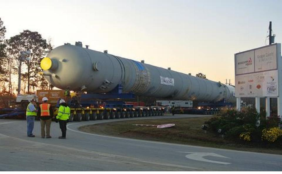
A hydrogen sulfide (H2S) absorber being delivered to the plant
