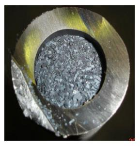
**Tube Blocked by Oxide Scales**
