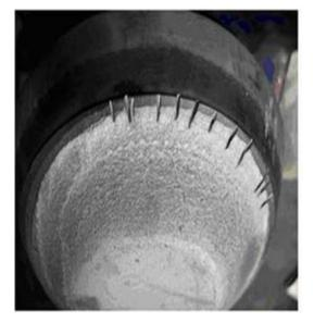
Turbine Blades Eroded by Solid Particles
