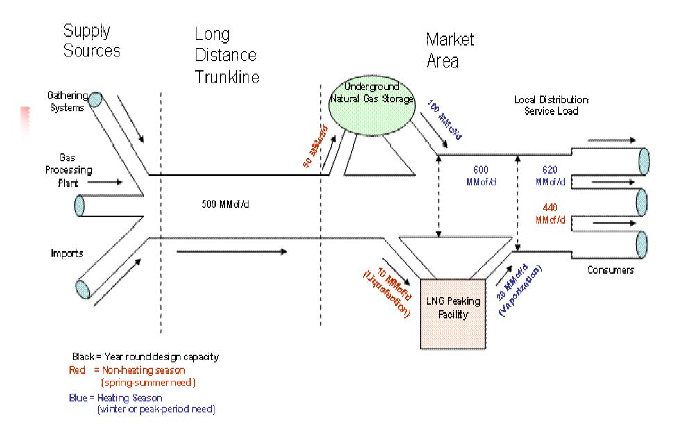
Note: MMcf/d = million cubic feet per day. Areas shown are not proportional to capacity volumes indicated. Other natural gas transmission pipelines may interconnect with and supplement the supplies of the mainine transmission or local distribution company in the market area to meet peak period demands.
